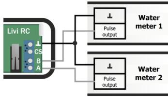
Connecting one water meter or one electricity meter to the sensor:
